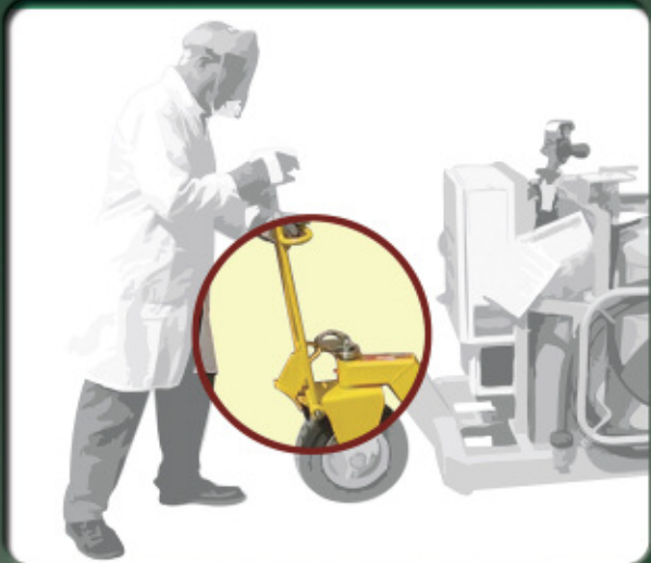
Position rig and apply brake
