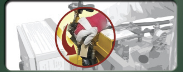
Open rig's nitrogen cylinders and, using donor regulator, charge in 250psi stages to a maximum pressure of 2500psi
