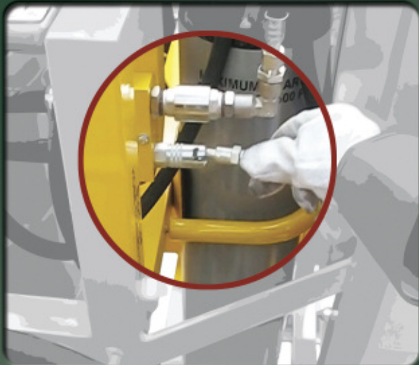
Connect blow-off hose to rig's nitrogen supply
